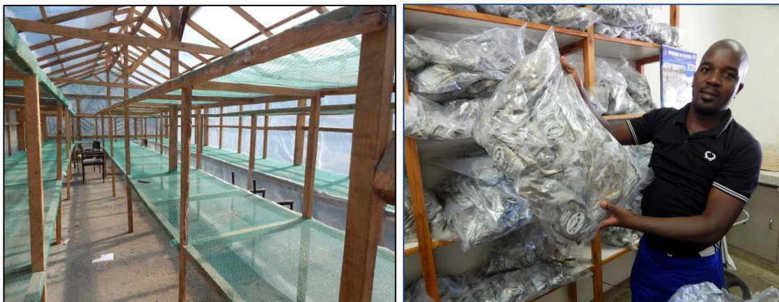
Photos 3 and 4. Solar fish dryer racks and packaged product. In the interior of the dryers, shelves or holding trays are fitted where the fish are placed to dry. The final product is packaged in 100 gram fish bags. (photo credit: James Tobey)
