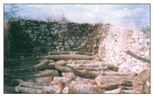
**Figure 2.5: Firewood logs in a Traditional Lime Kiln (Lirangwe, Blantyre)** *Source: MIRTDC, Blantyre*
