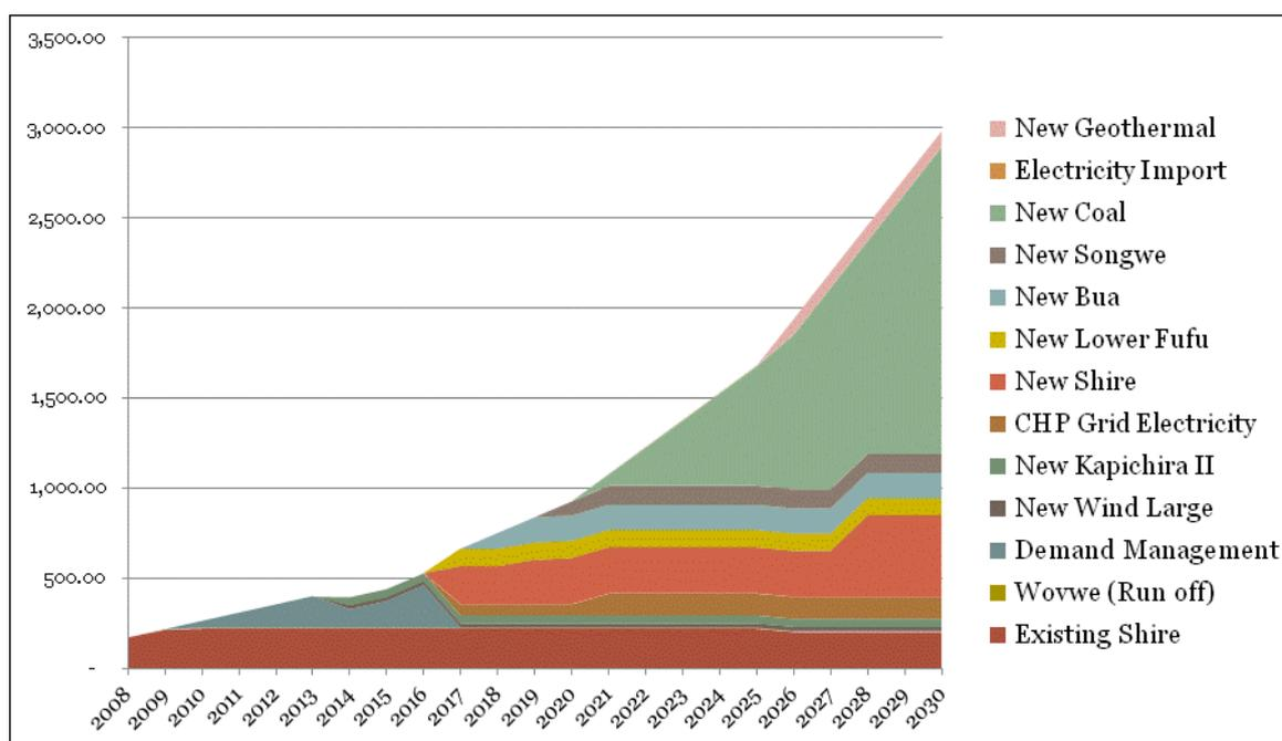
**Figure 3: How Centralised Electricity is Supplied (MWyr)**
