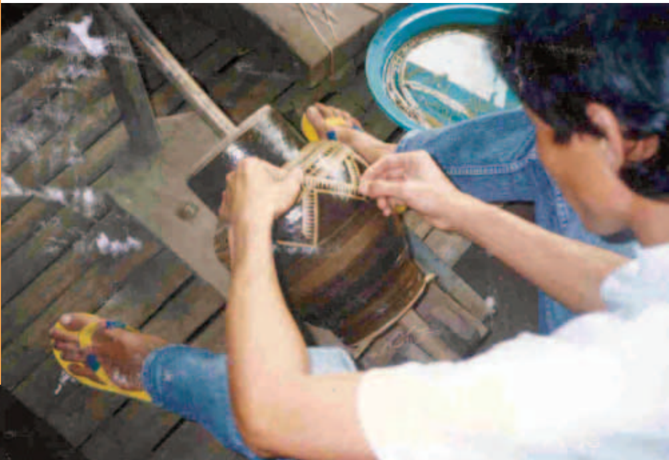
Brasswear co-operative member finishing the application of resin in mould, Tugaya, Philippines © ILO INDISCO
